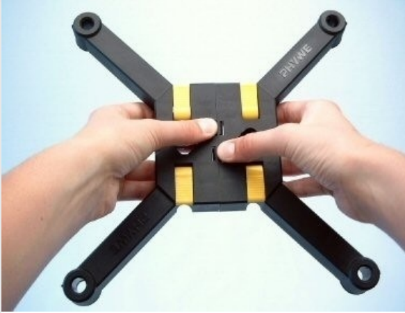
Disassembling the tripod base
